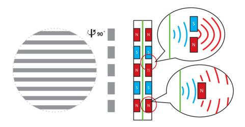
Unlike the sound waves created by a conventional magnet, the special shape of stealth magnet of ARYA UNVEILED enables the waves to pass through the magnets without generating interference.
