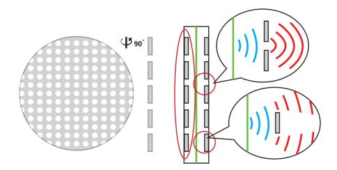
Degradation of sound quality in a conventional planar magnetic headphone is caused by the magnets getting in the way of the sound wave.
