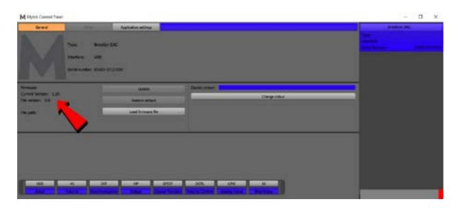
• The firmware can be updated by using USB2 port and Mytek Control Panel application. It does not require installed USB2 driver (PC). To download the current firmware please visit: www.mytek.audio
